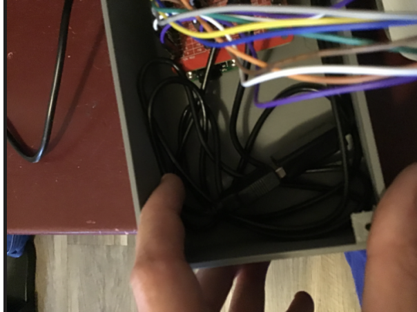
Figure 6.3.11: Example of Tucking Excess Cabling
